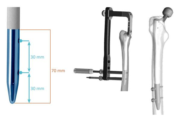
Remove the proximal drill bit and use the threaded pin size gauge to determine the length of the threaded pin needed. The threaded pin is then inserted with the short H5 screwdriver (for stem locking). Continue turning the screw until the mark on the screwdriver is flush with the drilling barrel.
